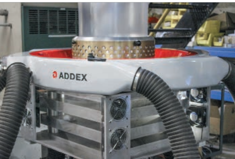
Addex's ICE unit is mounted between the die and air ring; the cooling elements are surrounded by an enclosure to improve bubble stability.
